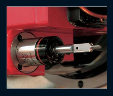
OCTOPUS 100 IS EQUIPPED WITH A 3D ELECTRONIC TOUCH PROBE WITH PROBING TIP MADE ACCORDING TO DRAWINGS AND CRASH PROTECTION PIN. THE PROBING SOFTWARE INCLUDES AXIAL AND RADIAL TOOL POSITIONING AND LEAD CALCULATION.
