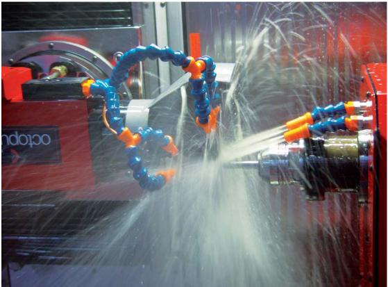
The kinematics of Octopus 100 is composed of 4 linear and 3 rotary axes assembled in two clearly defined areas of the machine base. Linear axes X, Y, Z and rotary axis B
