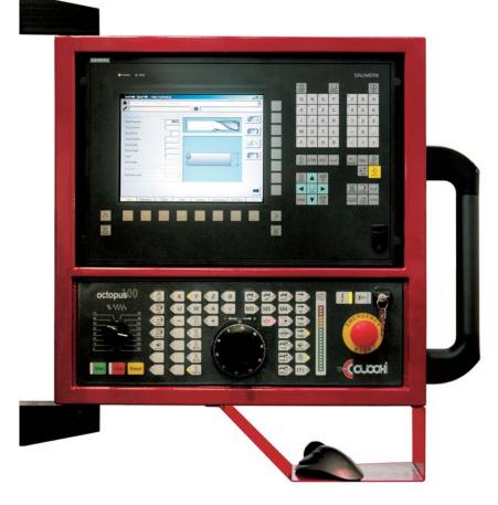
The positionable console contains a modern and efficient SIEMENS SINUMERIK 840Di numeric control that integrates our OCTOSOFT programming software.
